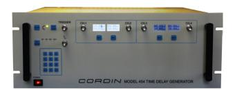
The Cordin Model 454 Time Delay Generator is a very reliable and robust delay unit. It will produce four channels of delayed output with delay ranges from 10 picoseconds to 999.99999 milliseconds. Delay values have an eight digit resolution. Pulse width of the output is selectable between 50 nanoseconds and 999.99 milliseconds.
