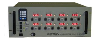
The Cordin Model 458 Time Delay Generator is a very reliable and robust delay unit. It will produce eight channels of delayed output with delay ranges from 10 nanoseconds to 99.99 milliseconds. Delay values have a four digit resolution. The full range of delays is covered by four range settings; 00.00 milliseconds, 0.000 milliseconds, 00.00 microseconds and 0.000 microseconds. Pulse width of the output is selectable between 1.0 microseconds and 100 microseconds.
