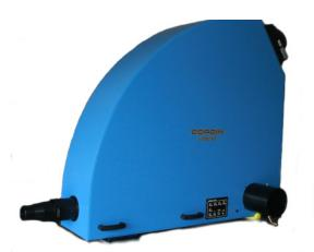
The **Cordin Model 510** high speed rotating mirror CCD camera is the world's fastest non-intensified digital imaging system. The Cordin rotating mirror technology provides significantly better image quality and a higher number of frames than is achievable with any other high speed camera technology.
