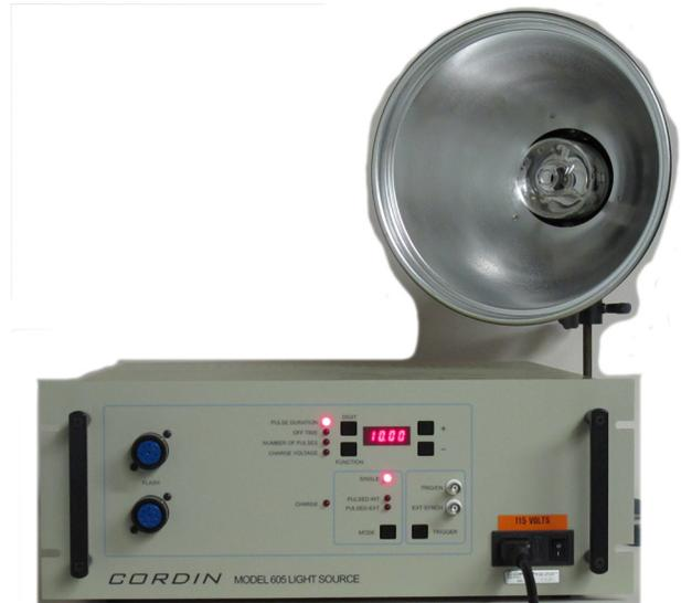
The **Cordin Model 605** is a high intensity xenon light source that is designed to give even intensity output during the full pulse duration. This is useful for high speed imaging as constant exposure can be maintained throughout the record. Conventional xenon strobe units will follow a modified R-C intensity curve with a relatively gradual rise and decay. The 605 is designed to have a rapid rise, maintain intensity across the pulse duration, and then have a rapid decay.
