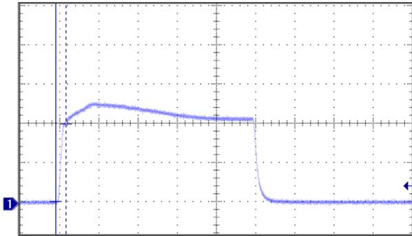
Model 605 pulse output - intensity over time
