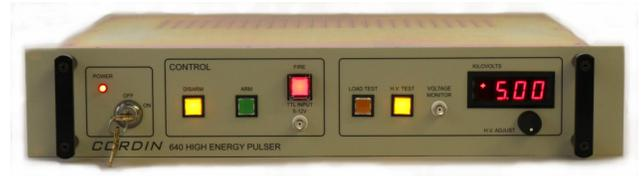
The **Cordin Model 640** High Energy Pulser is a highly reliable and accurate firing unit that has been a standard for initiating explosive and other events for decades. It is capable of producing pulsed output of up to 10 kV.
